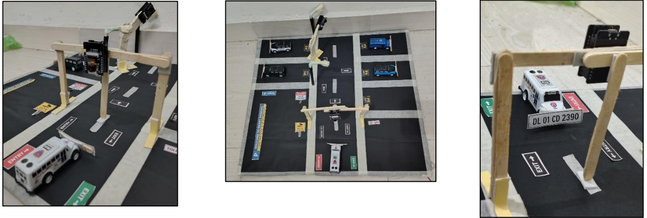
Fig2. Experimental setup of the parking slot detection model
