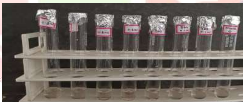
Figure 3: EPS Analysis using phenol-sulphuric acid method at 480 nm before incubation.
