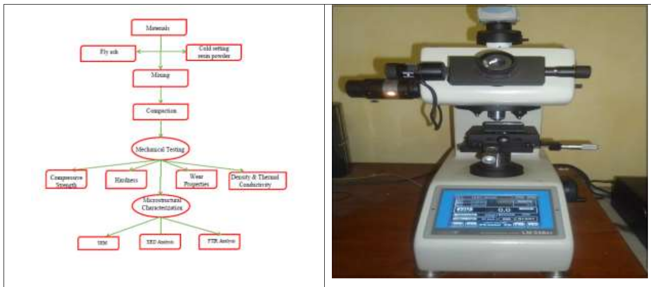
Fig. 3.2 Experimental Procedure Flowchart and Micro Indentation Hardness Tester (Leco LM-248AT)
