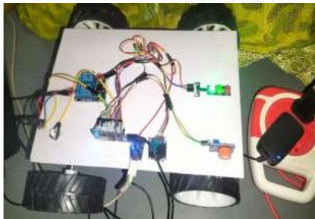
Fig . 4 Hardware Prototype Setup of the Proposed Real-Time Drowsiness & Distraction Detection System.
