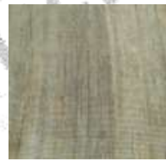
Fig. 7 Back view of the cured composite, 3 mm composite
