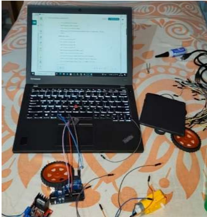
Figure 3.Voice-controlled wheelchair circuit setup during testing.
