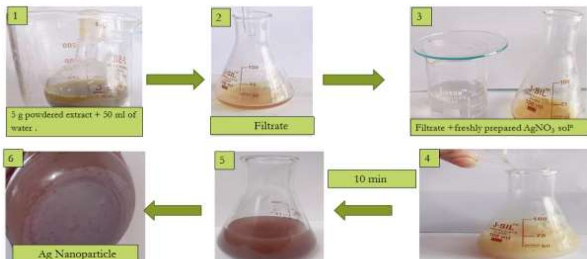
Figure 2. Step by step synthesis of Ag nanoparticle from SL plant extract
