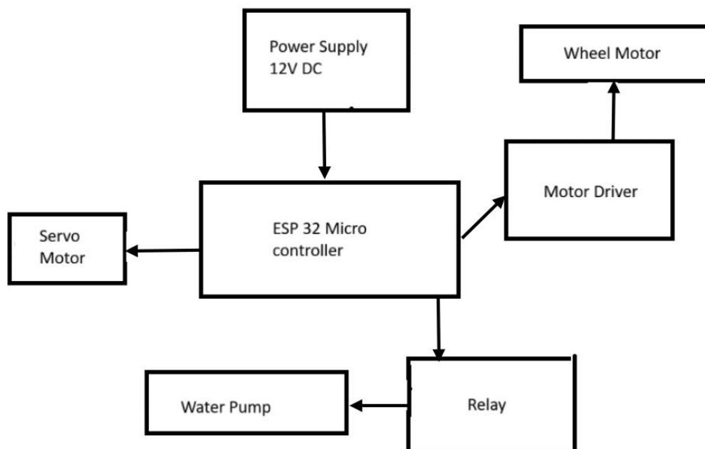
1. The fundamental component of the system that regulates movement and spray functioning is the Control Unit (ESP32).
