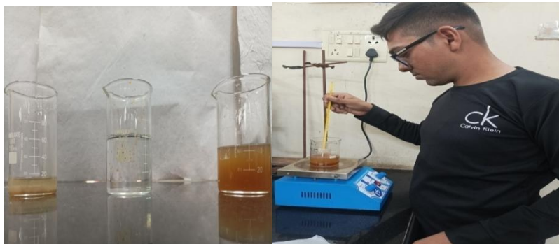
Fig 2.2.3 : Separation of Aqueous and Organic Phase
