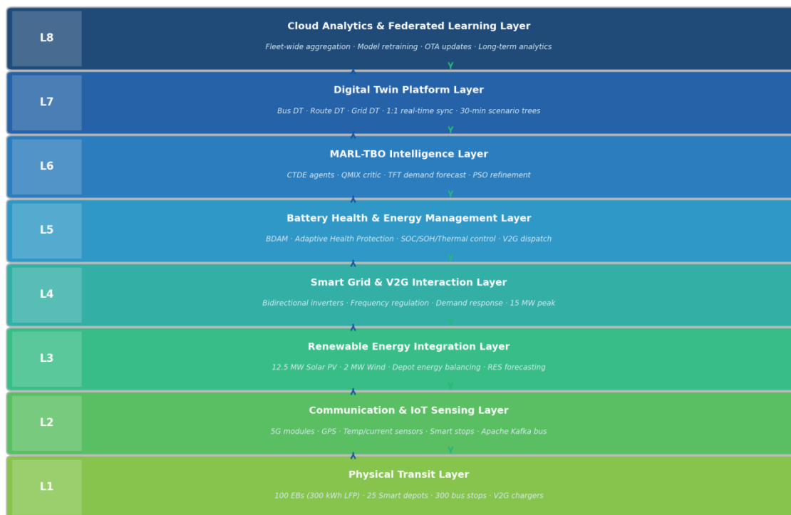
Figure 1. Proposed eight-layer Smart Transit System (STS) architecture showing hierarchical control layers and bidirectional real-time data flows between the Physical Transit Layer and the Cloud Analytics Layer.
