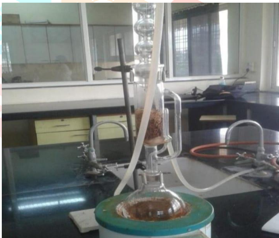
figno.10 Soxhlet extractor
