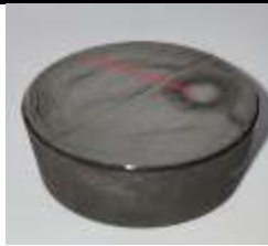
Fig. 3 Surface section where the OES is done.
