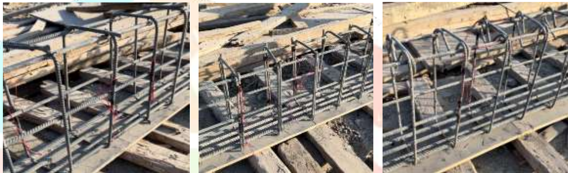
Fig. 6 Configuration of strain gauges for the stirrups, bott. RFT, and long RFT.
