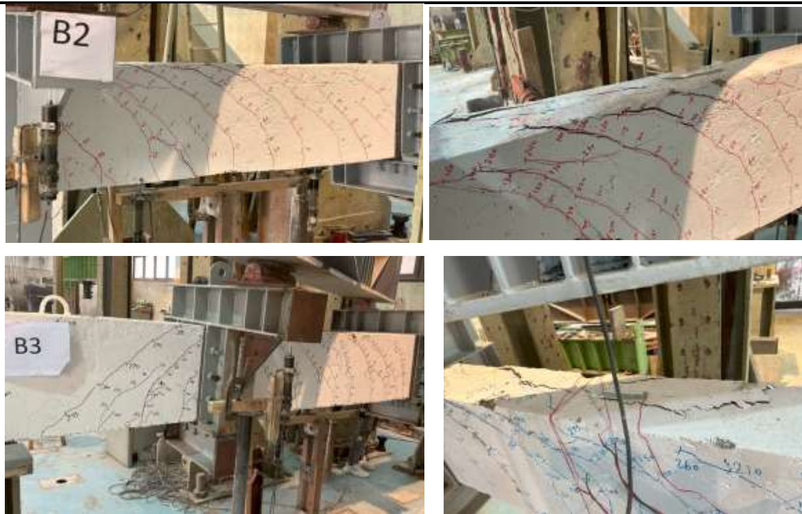
Fig. 7 Failure characteristics and Crack Patterns for tested specimens.
