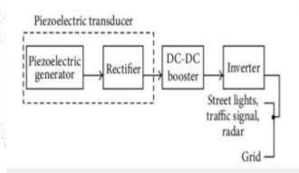
PIEZOELECTRIC ROAD: The roads which produce electricity by application of mechanical energy when vehicle moves over the road, those roads are called as piezoelectric roads
