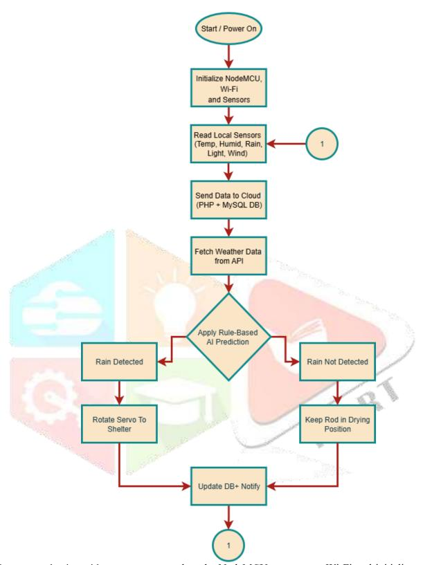
The process begins with system startup when the NodeMCU connects to Wi-Fi and initializes all sensor modules. After that, the microcontroller monitors the data from the temperature sensor, humidity sensor, light sensor, wind sensor, and rain sensor.
