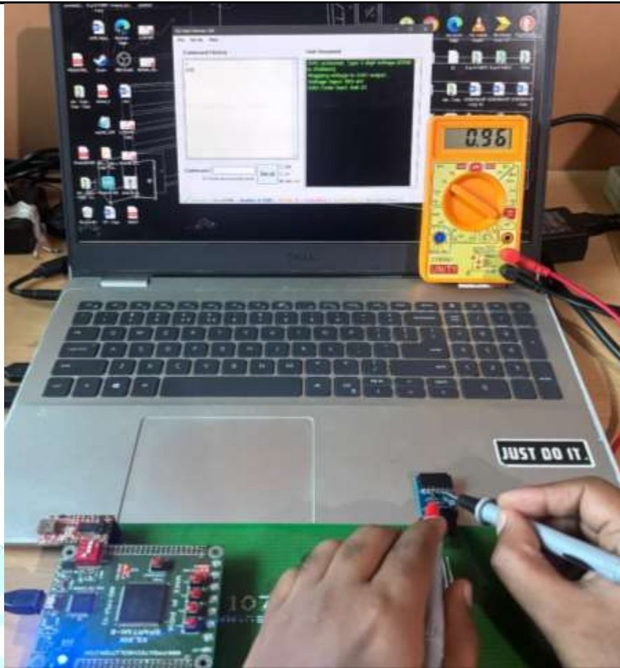
Figure 15. Demonstrates the input of 100 (representing 100 mV). The multimeter reading for this input was approximately 0.96 V, closely matching the expected theoretical output (minor deviation attributed to loading effects or absence of a buffer).
