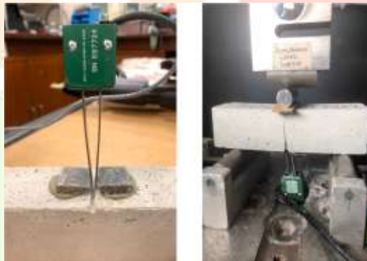
Figure 8: (a) The beam with thin metal bars attached (b) the 3-point bending test apparatus with the CMOD clip gauge connected
