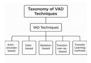
Figure 1: Categorization of neural network-based video anomaly detection approaches.
