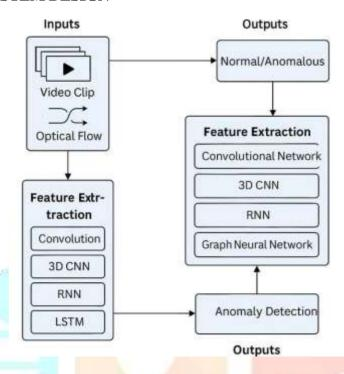
Figure 2: Architecture of the proposed neural network-based System for video anomaly detection
