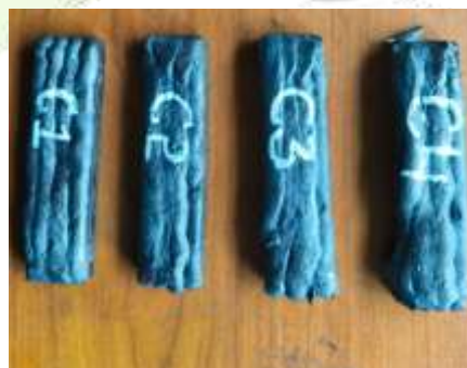
Fig 2: Hardfacing samples by MIG welding
