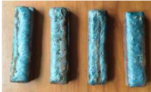
Fig 1: Hardfacing samples by SMAW welding
