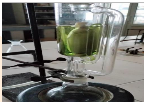
Figure No. 5.1: Soxhlet Extraction of Aloevera
