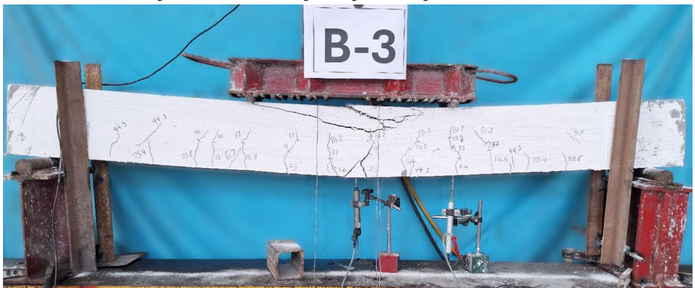
Figure 12: Concrete crushing and intact steel–concrete bond in beam 3 with lipped flange interlock.
