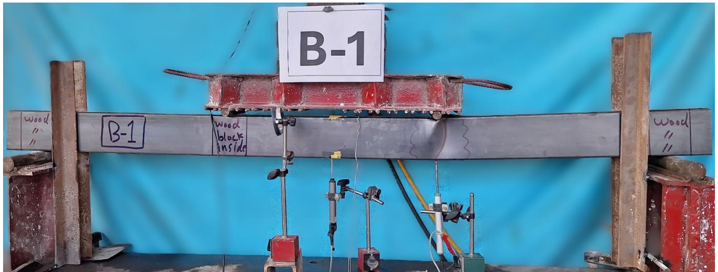
Figure 10: local buckling observed in beam 1 following flexural failure
