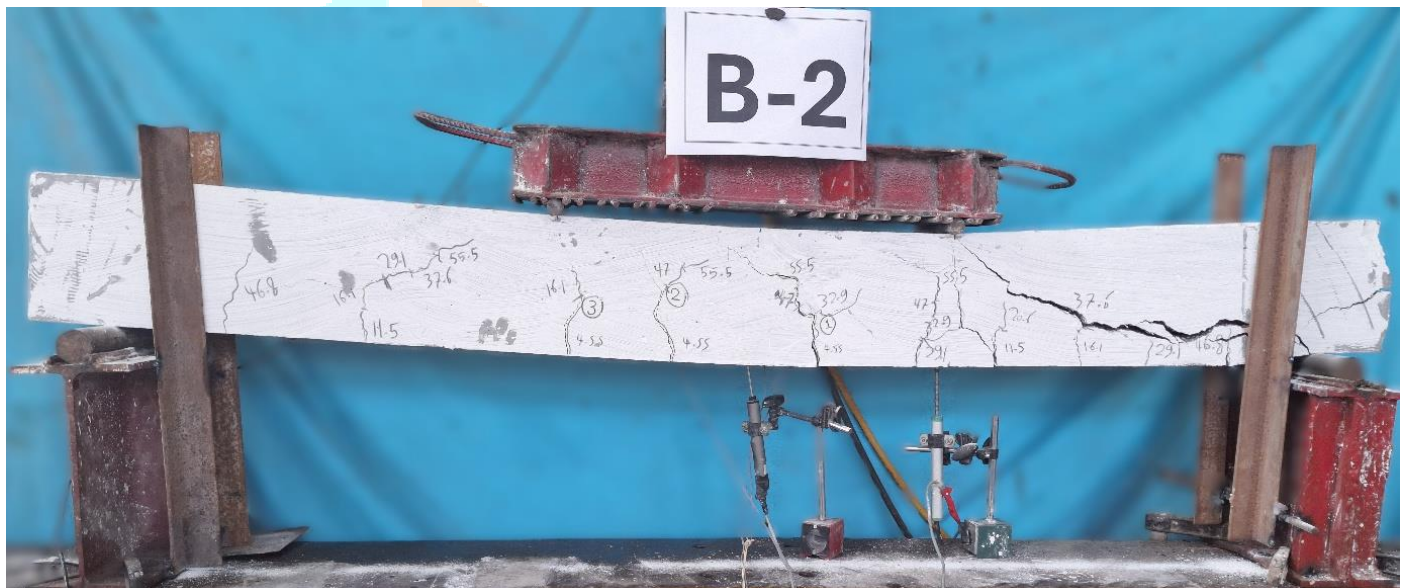
Figure 11: Interface debonding and diagonal cracking in beam 2 under load.
