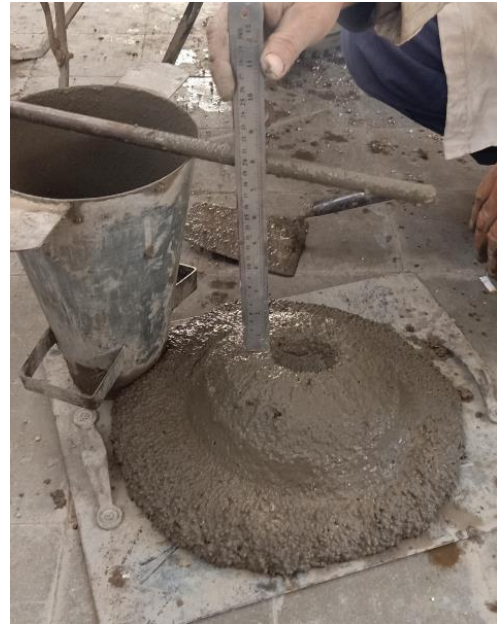
Figure 6: Fresh EPS-based lightweight concrete in slump test showing self-compacting consistency.
