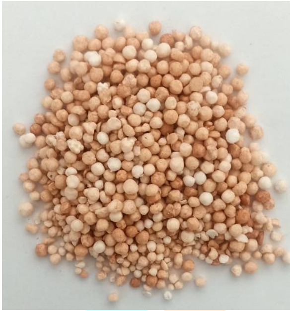
Figure 5: Recycled expanded polystyrene (EPS) beads used as lightweight aggregate in the LWC mix.
