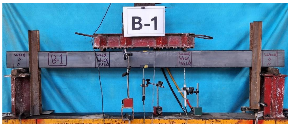
Figure 8a: Beam 1 under four-point bending test setup.
