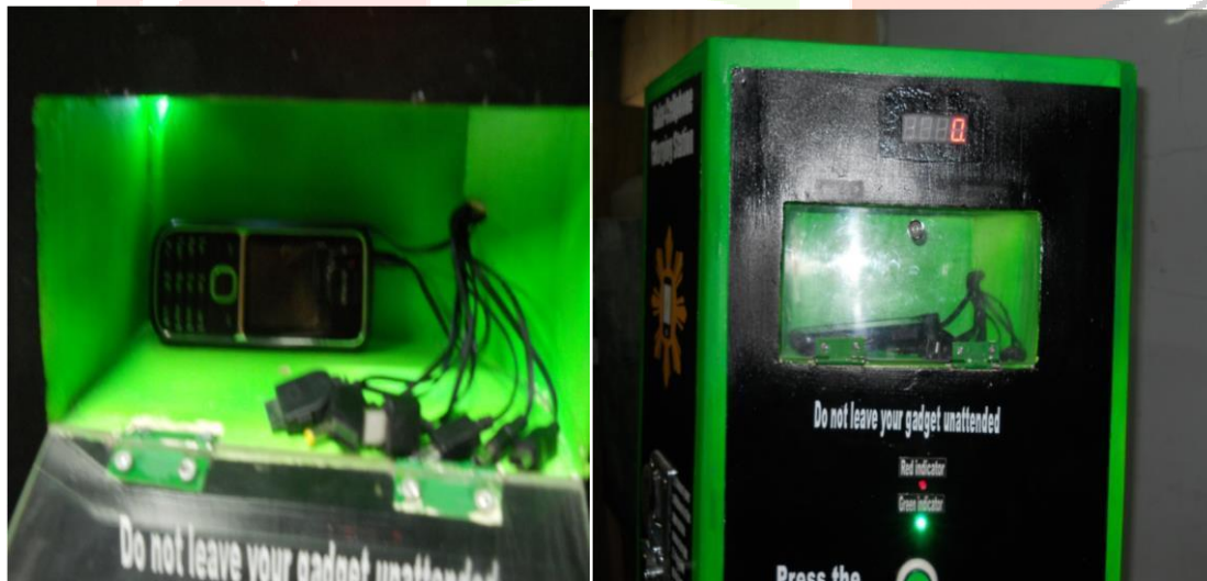
Figure 6. Cell phone charging compartment (the unit is provided with two compartments).
