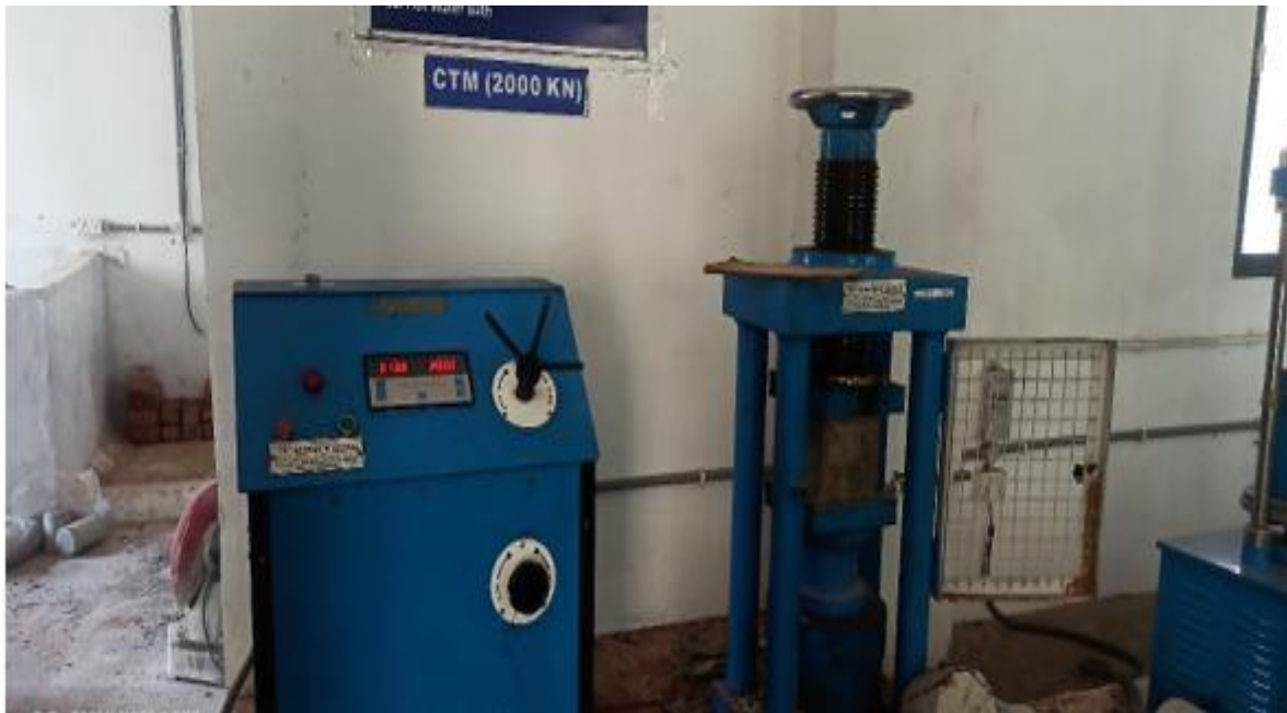
Figure 4.1: Compression test of concrete cube
