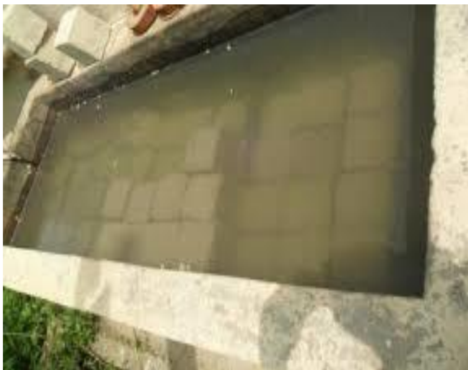
Figure 3.4: curing concrete cubes
