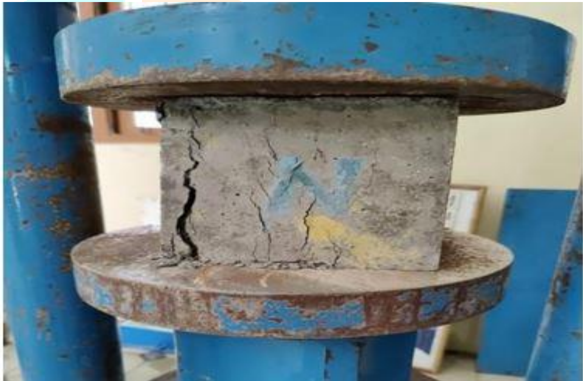
Figure 4.1: Compression test of concrete cube
