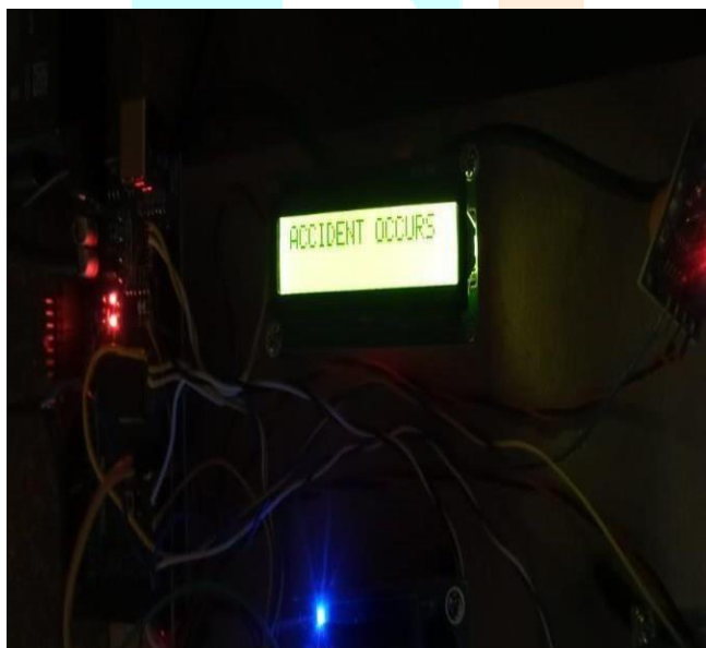
Fig 5.5. Accident Occurs Indication
