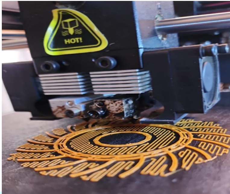
Figure 8: 3D Printing the cooling fan.
