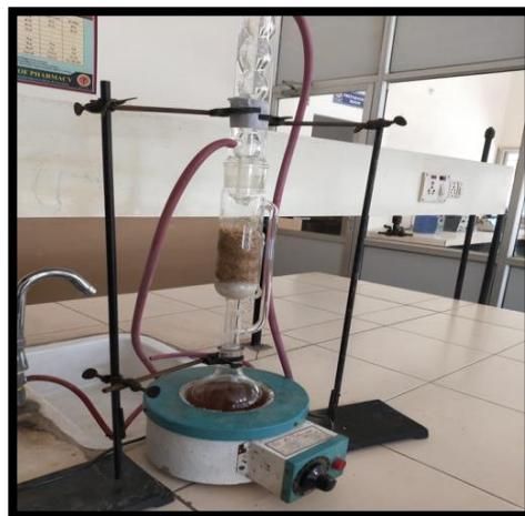
Fig.no.5. Soxhlet Extraction Method.
