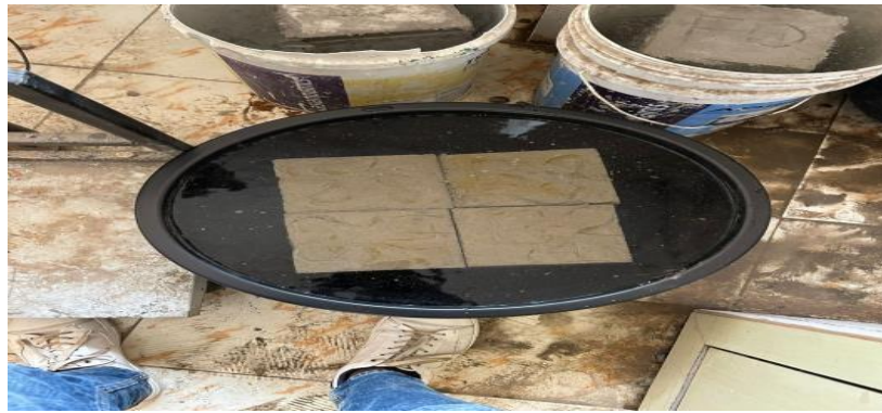
Curing of cubes
