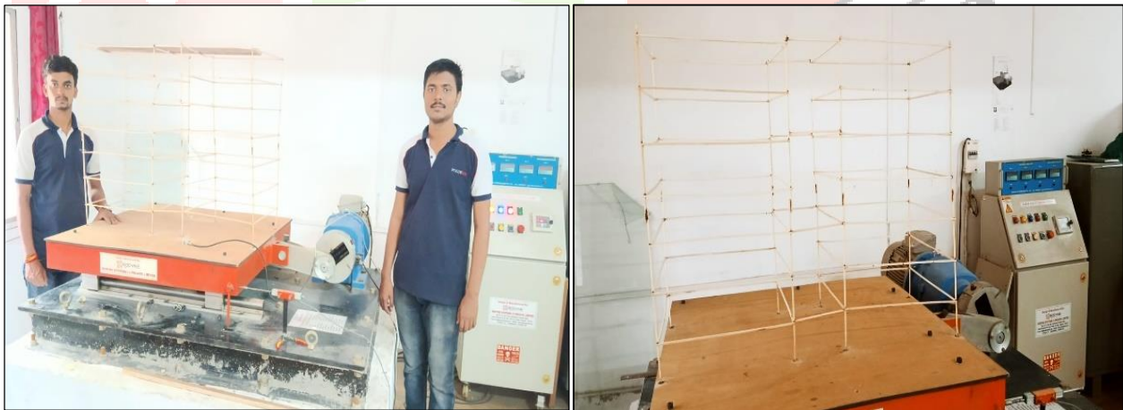
G+7 Building With Retrofitting Solution Model After Testing Figure no:-9
