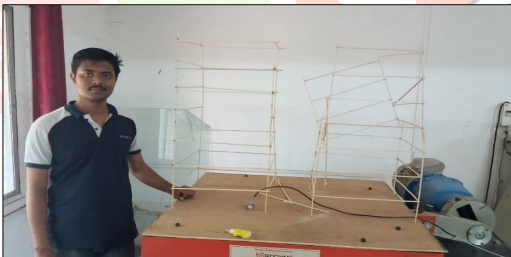
G+7 Building Without Retrofitting Solution After Testing
