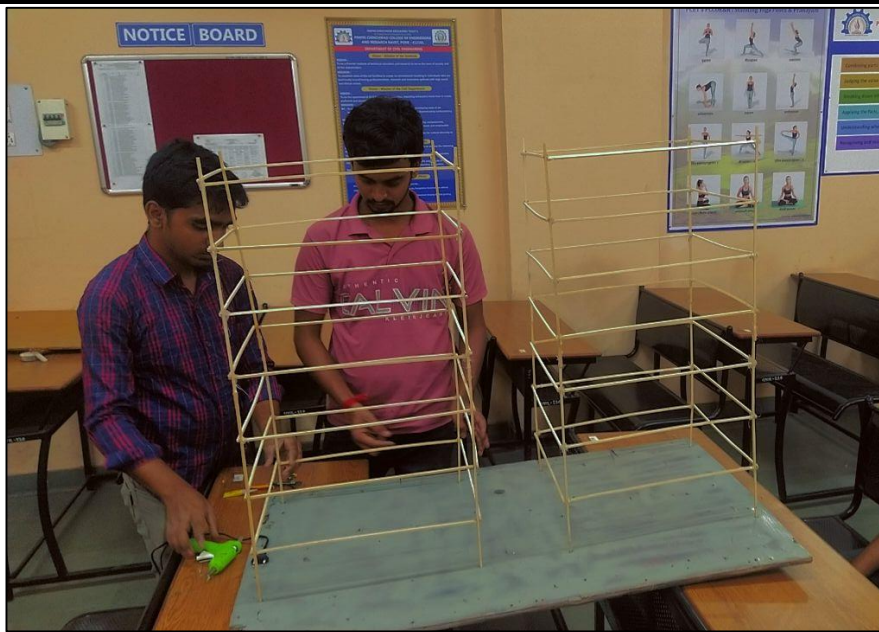
G+7 building Without retrofitting Solution before testing
