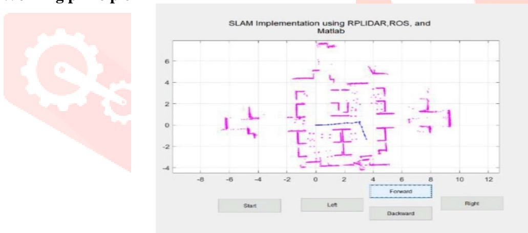
Fig. 3. The output obtained by the robot using SLAM algorithm -2D Map
