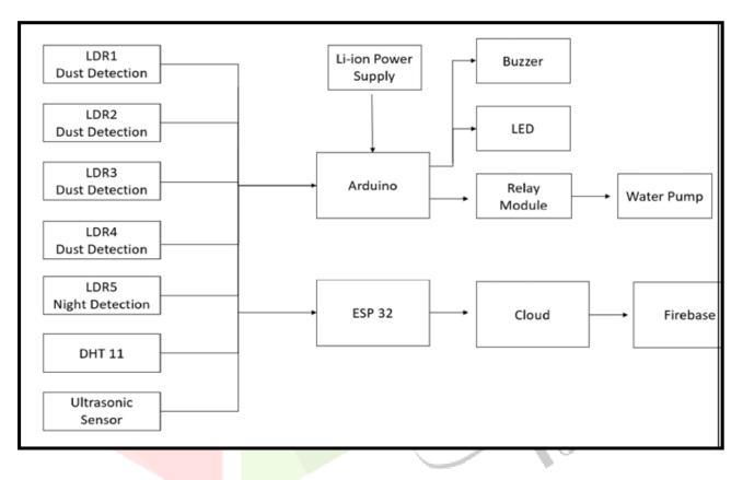
The proposed dust detection system uses four LDR sensors to measure the analogue value of a 10k resister attached to the panel. The intensity of the LDR sensor is affected whenever dust is deposited on the panel, and we assess the amount of dust deposited on the panel based on that intensity.
