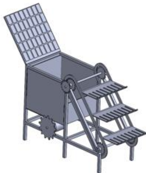
Fig 5 - Automatic Drain Cleaning System (3D)
