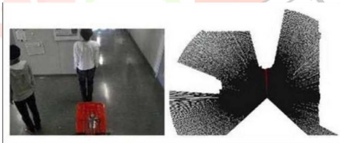
Figure 2: Example of Data Obtained from the Laser Range Sensor
