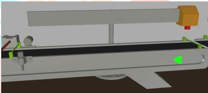
Figure 13: Sorting conveyor for sorting and distribution machine.
