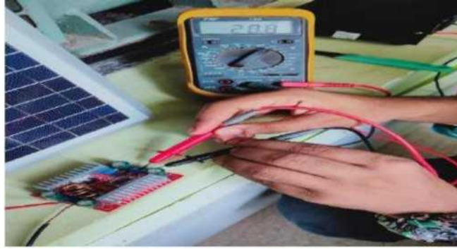
Figure 3.1.8: Output voltage test of DC-DC boost converter with multimeter
