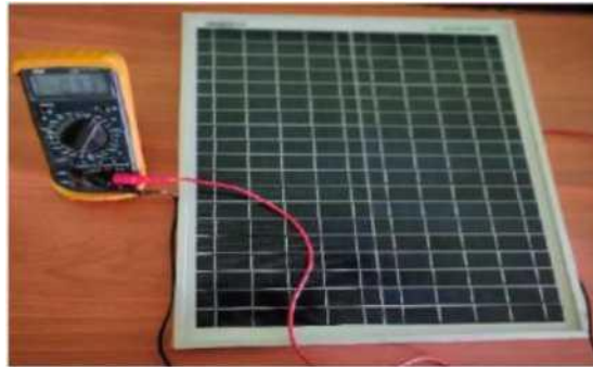
Figure 3.1.5: Open circuit voltage test of solar panel with multimeter
