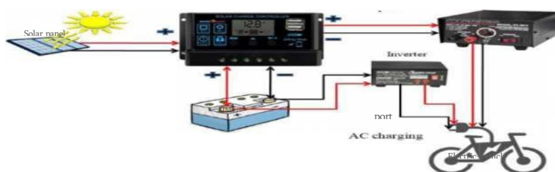
Figure 3.1.4: Block diagram of solar charging station
