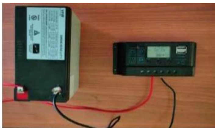
Figure 3.1.6: Output Voltage Test of Battery with Solar Charge Controller
