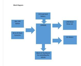
Fig. 1. Block diagram of the system
