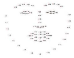
Eye Aspect Ratio [EAR]: The Eye Aspect Ratio (EAR) serves as a metric to detect both eye blinks and winks. When the eve is closed, the EAR value decreases, falling below a predefined threshold. Conversely, an open eye corresponds to an EAR value surpassing the threshold.
