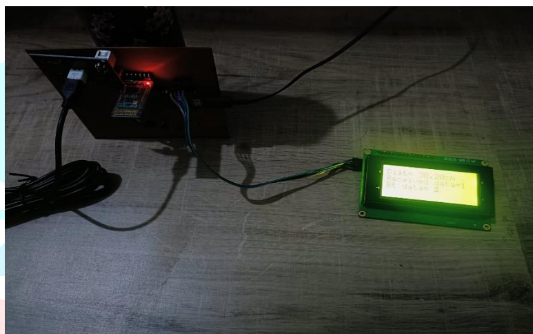
Fig. 4. Bluetooth Data is Received through IR signal
