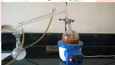
Figure 2 Extraction of whole cumin using distillation flask.
