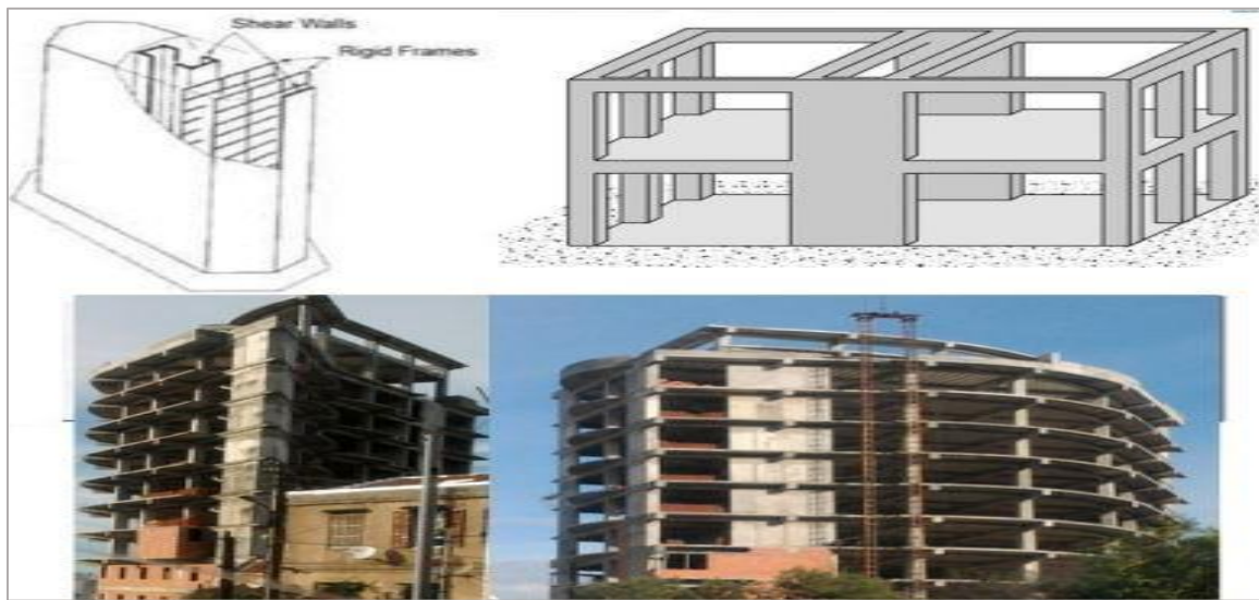
Figure 4 wall frame structure
