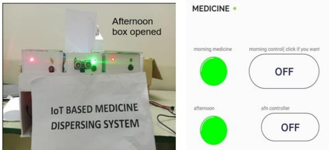
Fig. 15 The box opens in between 1.00 PM and 1.30 PM to enable user to take medicine and when medicine taken ,the status is updated in the Blynk Interface
