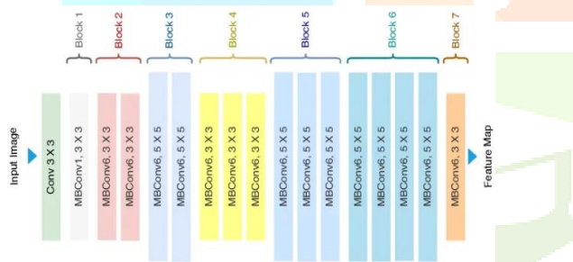
Fig 5: Efficient Net Architecture
