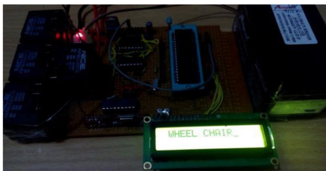
Fig 1: Receiver circuit of wheel chair with control unit.
