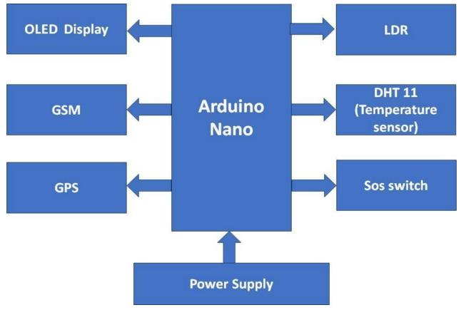
**ARDUINO NANO :** The Arduino Nano is a compact microcontroller board based on the ATmega328P chip, which is the same microcontroller used in the Arduino Uno. It's one of the smallest members of the Arduino family, making it suitable for projects where space is limited.
