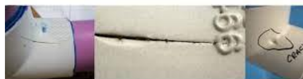
Cyclic Fatigue Failures
