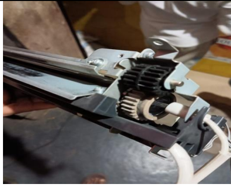
Figure 1: Fiber gears within a printer It is subjected to wear failure.
