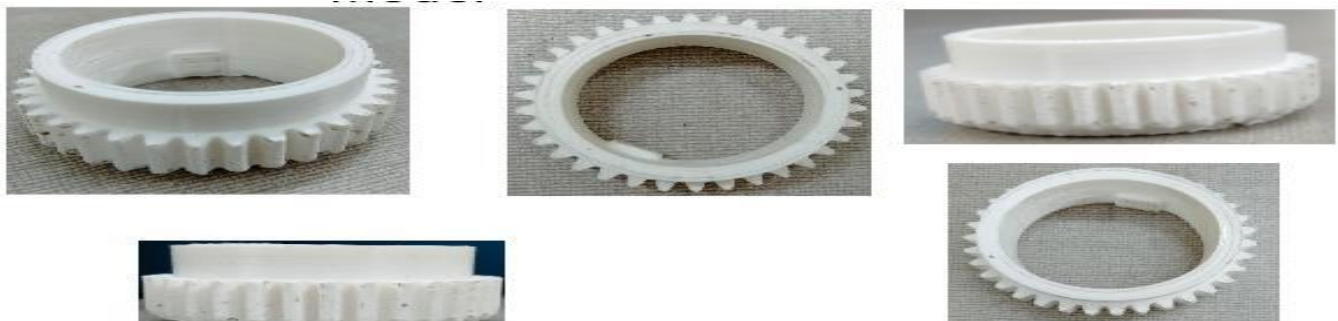
Figure 12: Modal prepare by using 3D printing machine based on dimensions
