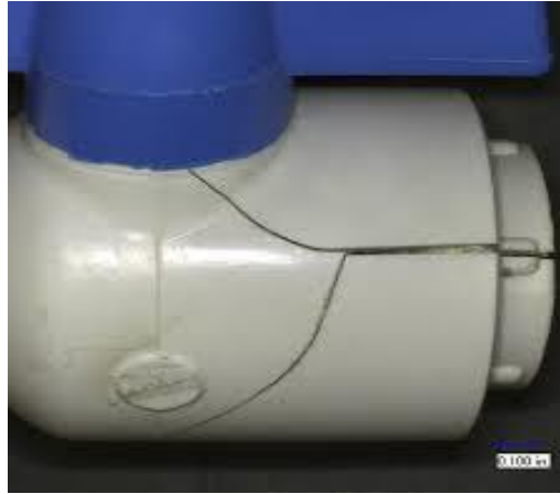
Figure 5: Plastic pipes may develop cracks.
