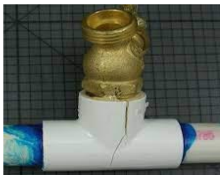
Figure 4: Failure at the joint
