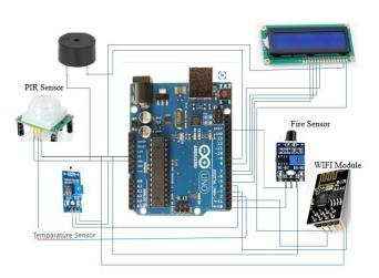
The above diagram represents the connection between sensors, buzzer, LCD.The analog pins are connected to the output pins.The vcc pins are connected to vcc pins.The Gnd pins are connected to Gnd pins.The sensors output pins are connected through analog pins.The four pins LCD is connected to analog pins.Gnd,vcc.The Arduino Board and Wifi Module are controlling the operations.
