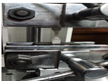
Figure 4.1 Tensile Test on UTM
