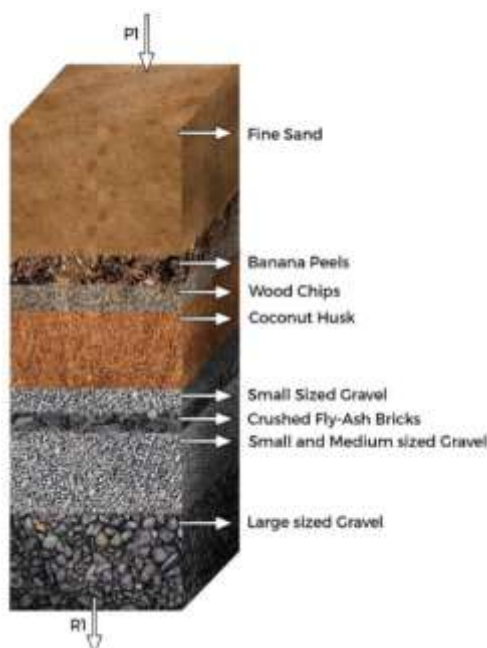
Fig. 01 - Filtration Assembly Fig. 02 - A schematic diagram of the mechanism of removing pollutants to supplement the system
