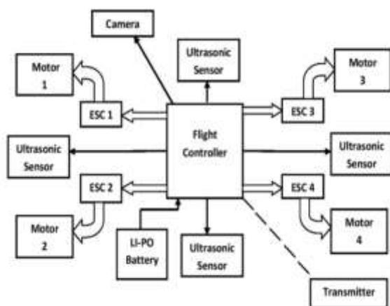
The hardware required for the proposed system includes an Flight Controller, Electronic Speed Controller, Brushless Motor, Transmitter and Receiver.
