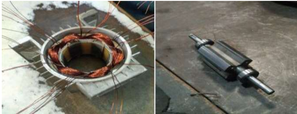
Fig.2.3 Actual Rotor & Stator with winding during assembly
