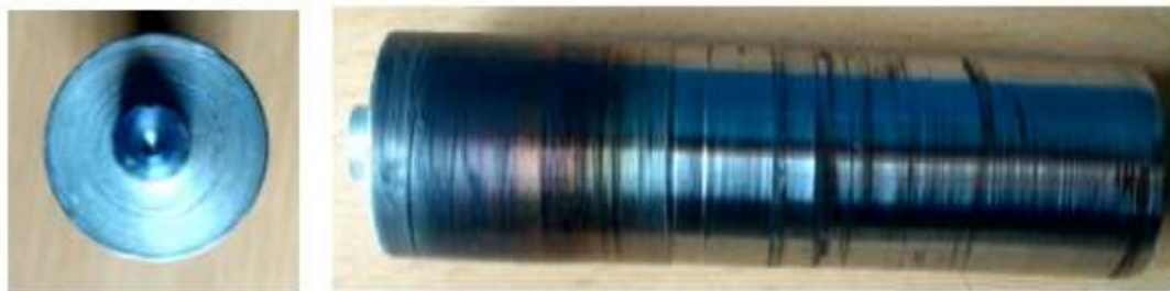
Figure 2.2 (a) Tool Pin & (b) Cylindrical Tool Used for Experiment
